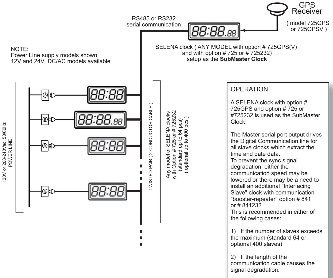
**Configuration using GPS as the Atomic time reference
