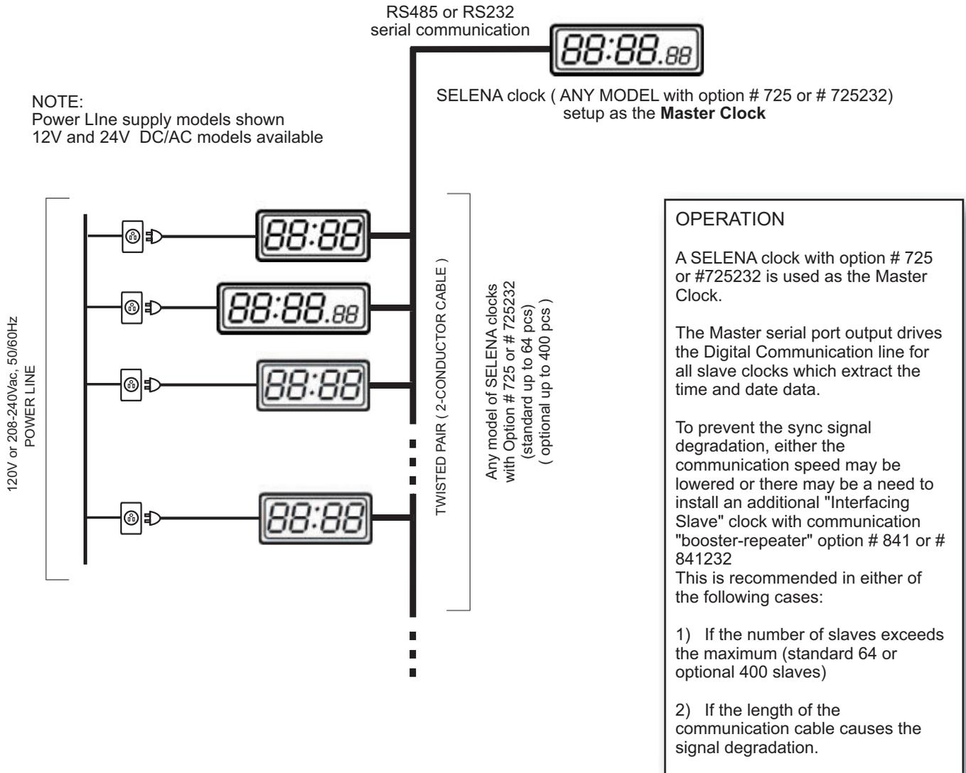
Configuration using RS485 or RS232 twisted pair
