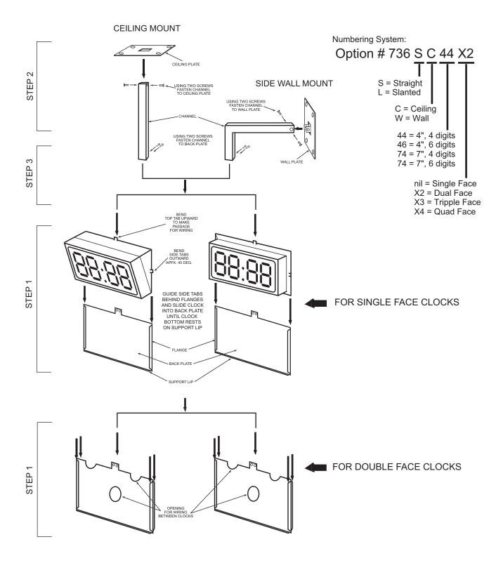
NOTE: INSTALL ALL WIRING BEFORE PROCEEDING WITH MOUNT ASSEMBLY
