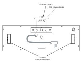
Short cord with flat plug shown Optional: Long cord or Screw terminal for power connection
